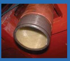
The thin wall liners have calibrated machined ends to fit exactly in the inner tube of the core barrel.
